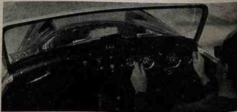
Instrument panel is neatly arranged, but gear lever is a shade too long, endangers driver's knuckles. Picture was taken from new space behind front seats.
