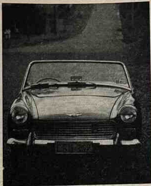
Bold front of the Sprite bears strong resemblance to Italian Innocenti Sprite. Winkers and parkers are combined.
