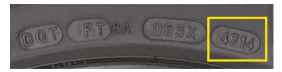
And how long will they last? Depending on which tyre company you talk to, the replacement age is between 6 and 10 years irrespective of the amount of tread that is left. This is because the rubber degrades over time as its exposed to sunlight, air temperature and even simply the air, and that's before you consider the surfaces that you've driven over and the effects of the pressure that you run you tyres at. From past professional experience, the results of old tyres can be catastrophic.
