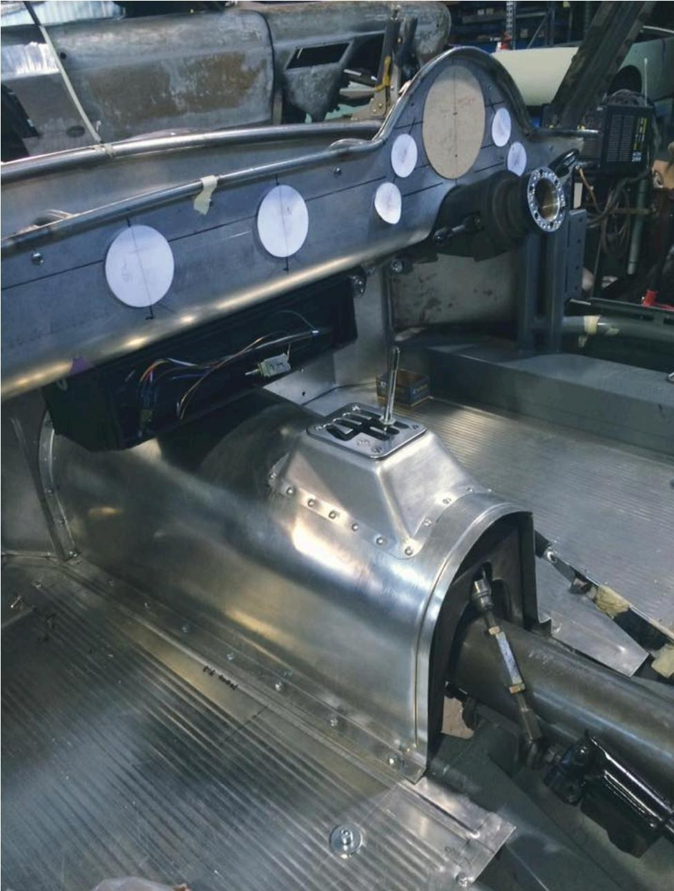
This vehicle will be road registered and will have some competition use, so has had roll bars, side intrusion bars and other safety items added to the body so it will meet all the safety standards for these tasks.
